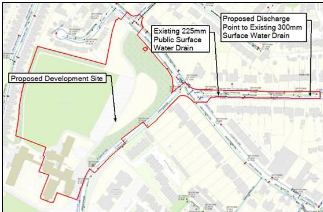
Figure 1.2 Existing Surface Water Drainage Infrastructure (Source: DBFL, 2021)
